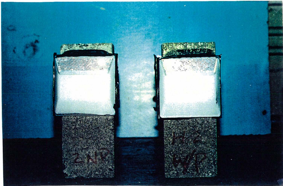
Figure 3.4.16 Shear failure of Hitack 2 on concrete. Left: Without primer; right: with primer
