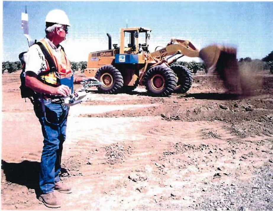
Figure 5.1 The front-end loader operated with the portable remote control unit
