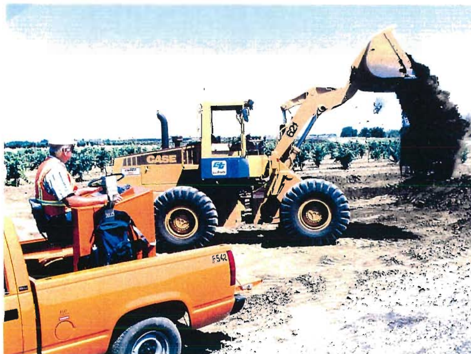
Figure 5.2 The front-end loader operated with the stationary remote control unit
