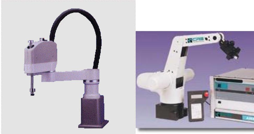
**Figure 2.2 - Adept 550 Horizontal and CRS Robotics A255 Vertical Articulating Robots**
