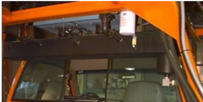
*Figure 2.20 Hydraulic Fluid Reservoir and Heat Exchanger*
