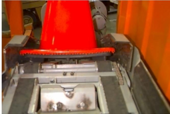
*Figure 2.13 Cone Positioned on Wing Section*
