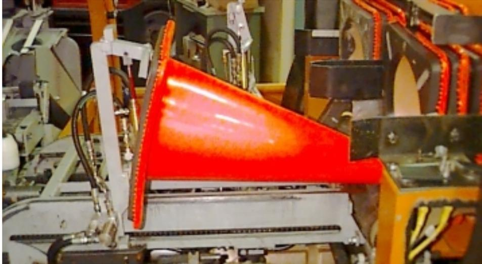
*Figure 5.23 Loss of Cone Retention by Gripper Assembly*
