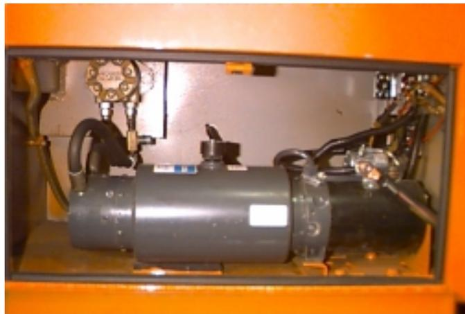
*Figure 2.6 Main Conveyor Belt Power System*
