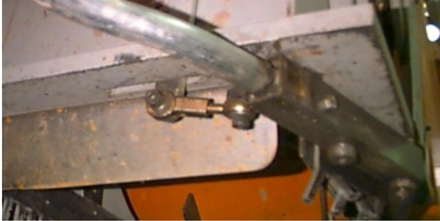
*Figure 4.20 Ball Joint Link of Secondary Funnel Folding Mechanism*
