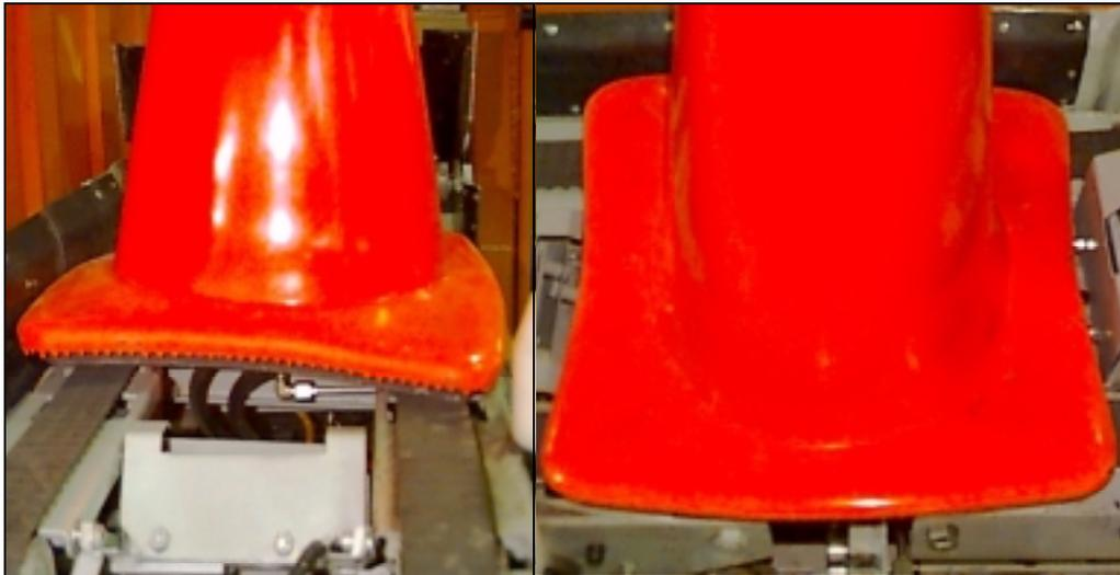
*Figure 5.24 Cone Deformation by the Gripper Shoes*
