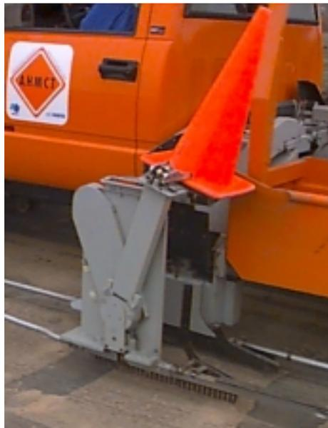
*Figure 4.16 Retrieval Arm, In Operation*
