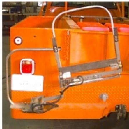
*Figure 2.17 Retracted Primary Funnel System*
