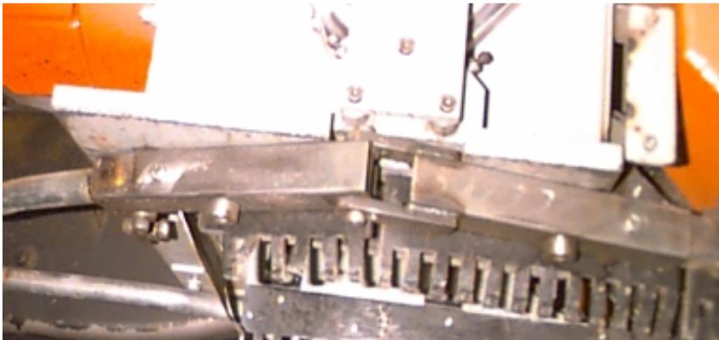
*Figure 4.19 Stowed Secondary Funnel Folding Mechanism*
