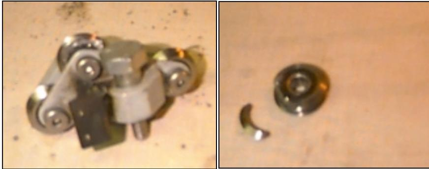
*Figure 5.25 Upper V-Wheel Failure on Cart Subassembly*
