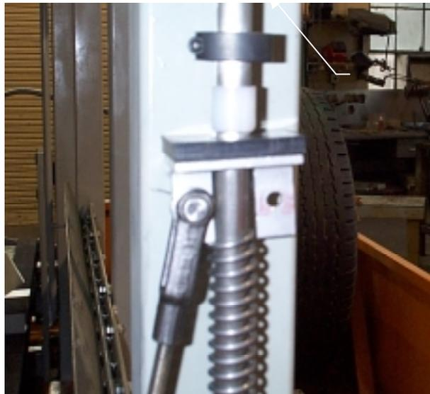
*Figure 3.16 Binding of Mechanism Slider*
