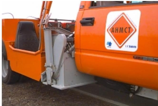
*Figure 2.15 Stowed Drop Box System (Right Side)*
