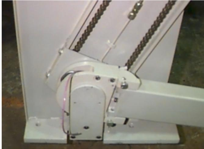
*Figure 4.15 Retrieval Arm, Rotational and Break Away Mechanisms*
