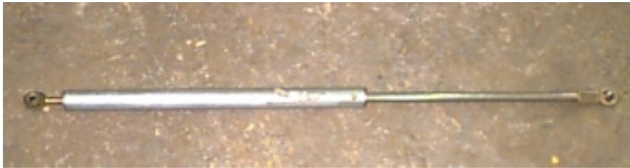
*Figure 4.21 Secondary Funnel Folding Mechanism Strut Link*
