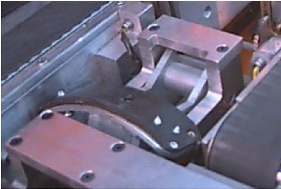
*Figure 5.1 Addition of Machine Screws to Gripper Shoes*
