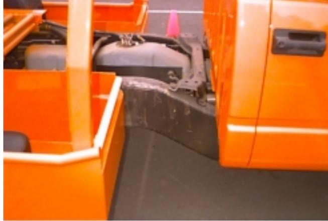
*Figure 2.2 Cone Truck with Rearward Moved Cone Body*
