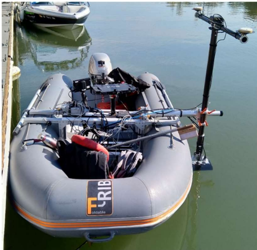
SM&I foldable boat with PicoMBES 120 sensor in water
